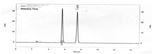
Fig.2. Chromatogram showing Retention Time (Rt) at 5.7min and 7.5 min for Sitagliptin and pioglitazone.
